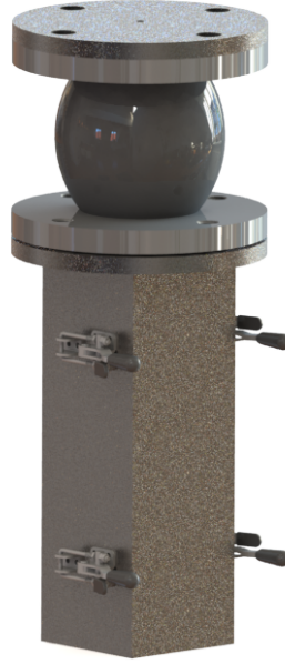
Figure 29. Finished rendering of cryochamber in desired materials. A flexible bellow can be observed on top.
