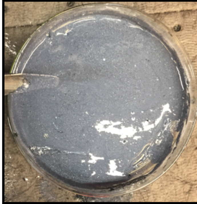
Figure 5. Completed PDMS-ZnO-CNT nanocomposite before it is combined with the scaffold.
